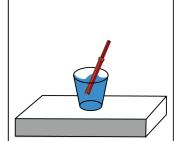
3. After completing hole, cool down in water and remove any material stuck in core. Do not force or overheat while in use.
